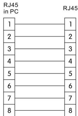
Figure 4.1.2 RJ-45 connector straight through connecting
